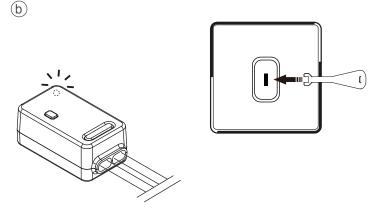
While the indicator on receiver flashes, press kinetic emergency key switch by using the key provided once to complete the pairing.
