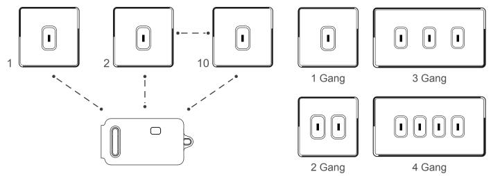
Max. 10 Kinetic Switches to pair ONE On / Off Receiver.
