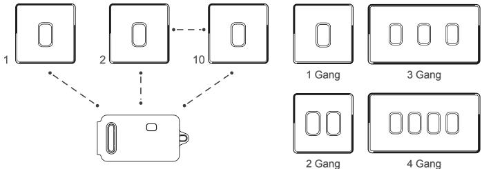
Max. 10 Kinetic Switches to pair ONE On / Off Receiver.
