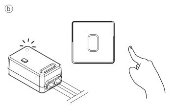
While the indicator on receiver flashes, press any key of Grid360 On-Off Kinetic switch once to complete the pairing.
