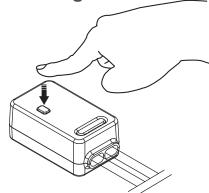
Press the Pairing Key for 3-4s, untill the RED indicator flash slowly. Order Controllers (On/Off) seperately.
