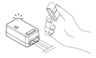
While the indicator on receiver flashes, press the Kinetic Fob switch ONCE to complete the pairing.
