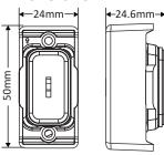
Power Source: Self Powered (Kinetic) Radio Frenquency: 433 MHz Switching Type: push on / off - emergency key switch (key tool inc.)
