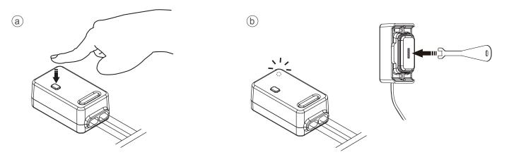
Press the Pairing Key for 3-4s, untill the RED indicator flash slowly. While the indicator on receiver flashes, press kinetic emergency key switch by using the key provided once to complete the pairing.
